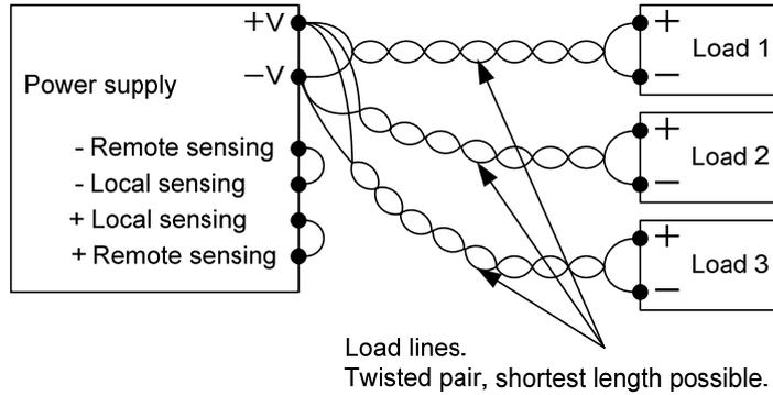
Fig.2-9: Multiple loads connection, radial distribution, local sense
