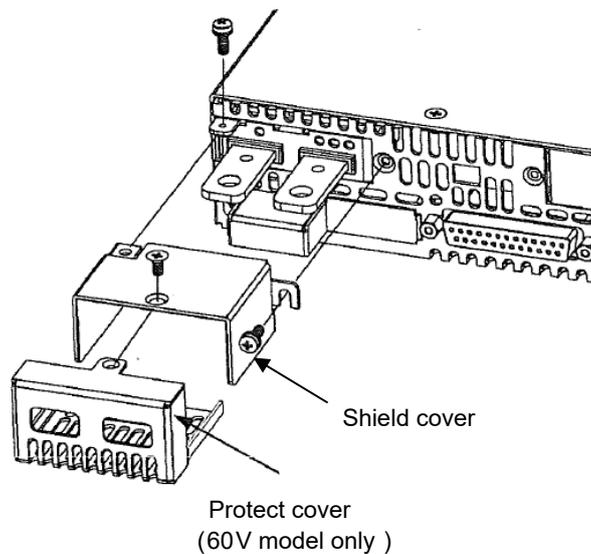
Fig. 2-3: Bus-bars shield mounting
