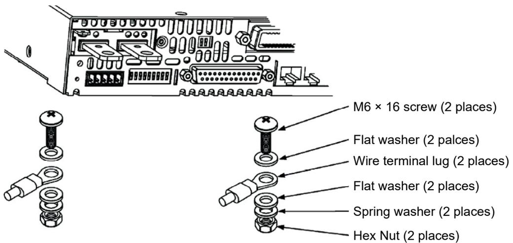
Fig. 2-2: Load wires connection, 6V to 60V models.
