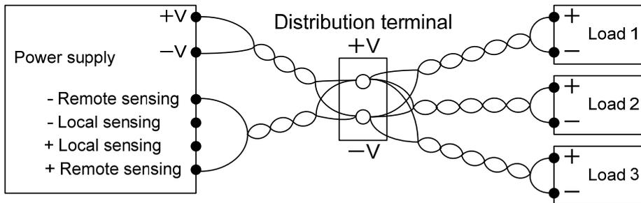
Fig.2-10: Multiple loads connection with distribution terminal
