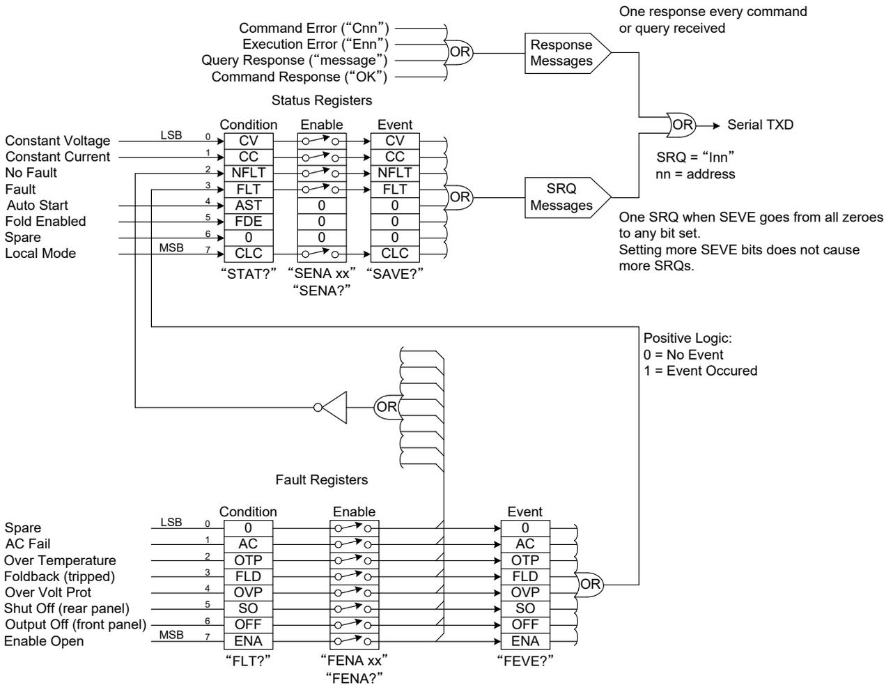
Fig.6-7: Status and Error Registers Diagram
