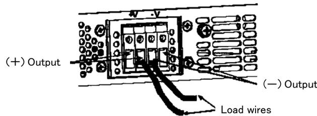
Fig.2-6: Load wires connection to the output terminal
