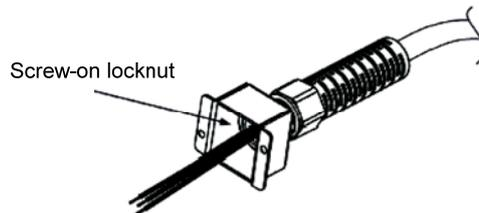
Fig. 2-1: Stripped wires installed in strain relief
