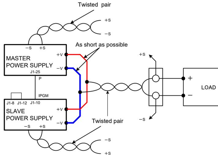
Fig.4-5: Parallel operation with Remote sensing
