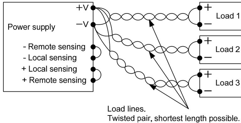
Fig.2-11: Multiple loads connection, radial distribution, local sense
