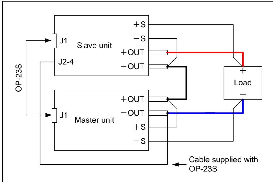
1. Connect the positive output terminal of the master unit to the negative output terminal of the slave unit, and connect the negative output terminal of the master unit to the negative side of the load. Connect the positive output terminal of the slave unit to the positive side of the load.
