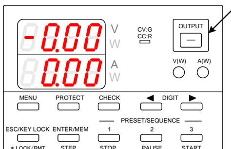
In the PS-A power supply unit, when the output of the unit has been turned on through the external contacts of the analog IF board, the OUTPUT key on the front panel can be used to turn the output on or off during operation. Thus, in case of an emergency where the power supply from the unit to the loads must be stopped, the power supply from the unit can be stopped without needing to turn off the power switch.
