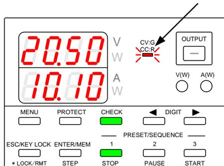
Turning the output on when CC priority mode is selected
