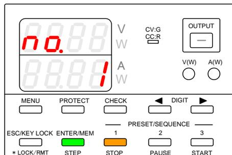
When a sequence program is stopped, the output will be turned off, even if the output is set to be on for the stopped step.
