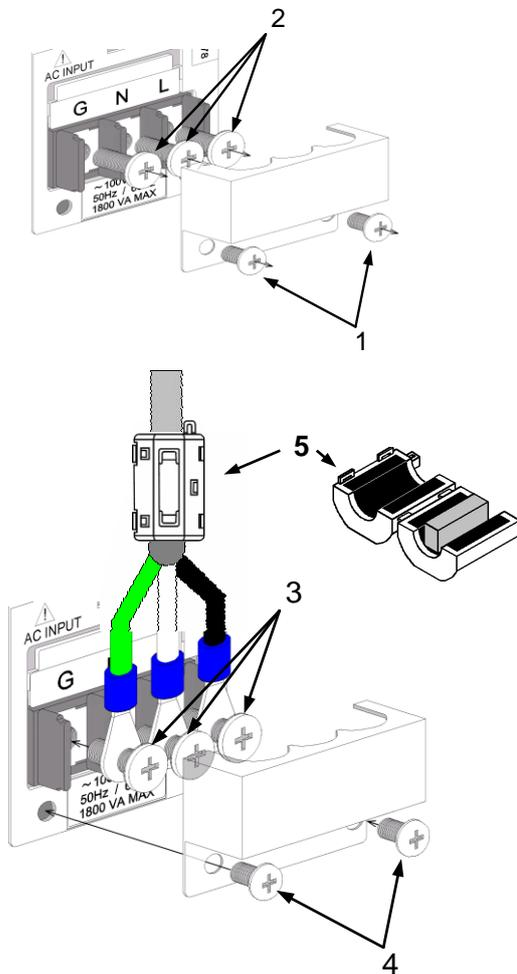
1. Unfasten the two screws that fix the AC input terminal block cover of the unit, and then remove the cover.
