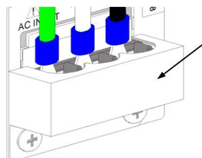
**Make sure to attach the AC input terminal block cover before using the unit.**
