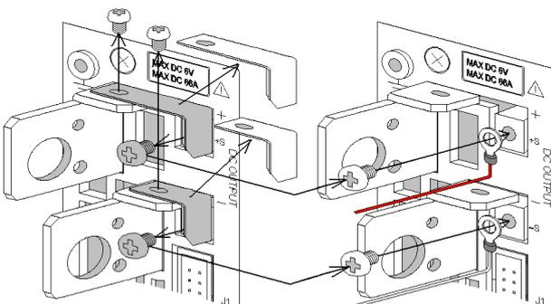
Remove the M3 screws (4 screws) from the positive and negative rear output terminals and the positive and negative voltage remote sensing terminals, and then remove the positive and negative shorting bars.
