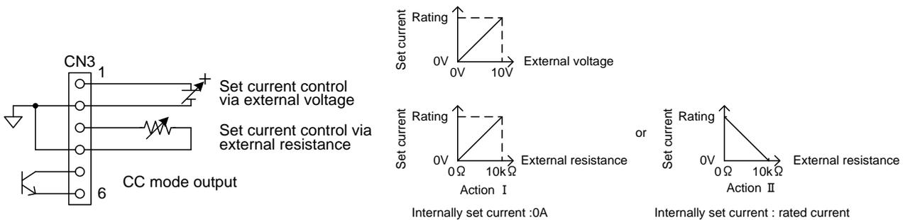
Set current control by external signal (Valid when pin No.7 of SW 1 is on)
