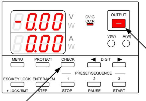
When the CHECK key is unlit, the output voltage and current are displayed.
