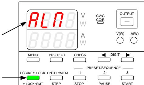
If the voltage indicator displays “ALΠ”, and the ESC key is lit in green, press the ESC key.
