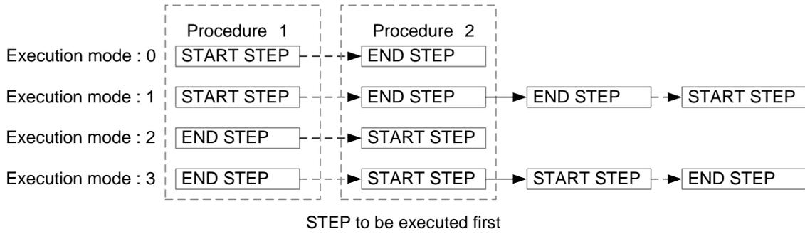
When the DIGIT keys ◀ ▶ are pressed to move to the next step or back to the previous step, if the execution time of the step to be executed next is 0 hr 0 min 0 sec 0 m.sec, the step will not be executed. The following step will be executed.
