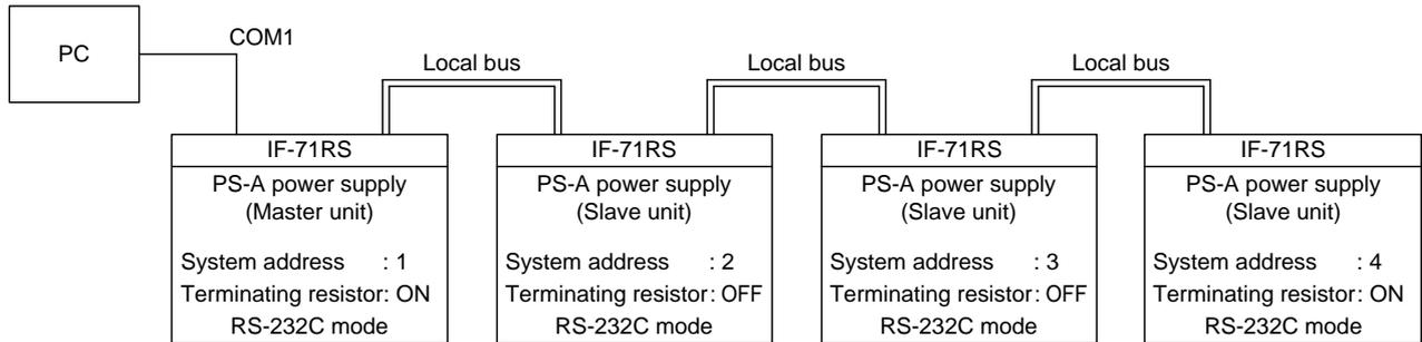
Slave units are designated by using the ADRS command to specify the system address numbers.
