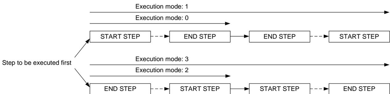
Automatic execution cannot start from a step that is in the middle of the sequence program.
