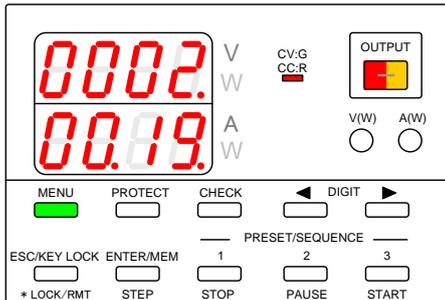
After the set time has passed, the OUTPUT key light goes out, and the output is turned off.
