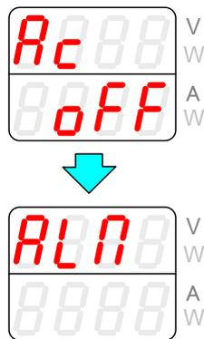
If the voltage and current indicators display “AC oFF” and then “ALΠ”, and the power switch has not been turned off, there may be a unit malfunction. Perform the following steps:
