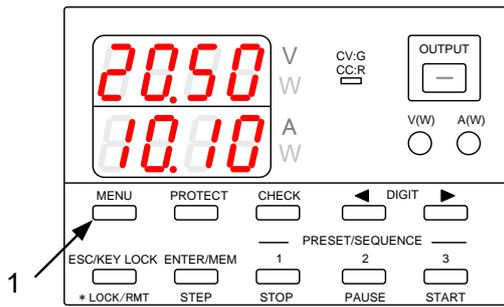
1. The discharge circuit does not activate if the MENU key is used to turn the HI-R function "ON" while the OUTPUT key is off.
