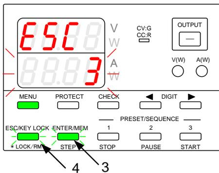
4. Press the green-blinking ESC/KEY LOCK key to exit.
