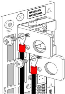
From the left side of the rear output terminals, attach the grounding cable to the M3 hole of one of the output terminals.
