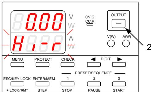
The voltage indicator displays the voltage of the output terminals.
