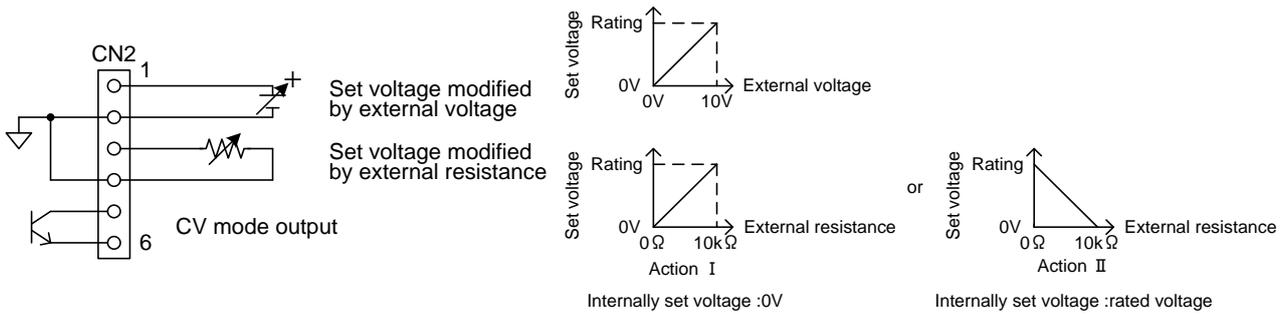
Set voltage control via external signal (Valid when pin No.4 of SW1 is on)
