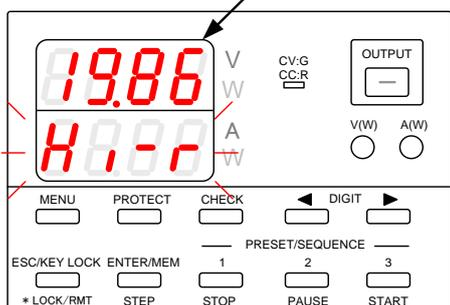
When the output HI-R function is "ON", voltage is applied to the output for a long time. If a capacitive load is connected, voltage is applied for an even longer period of time.
