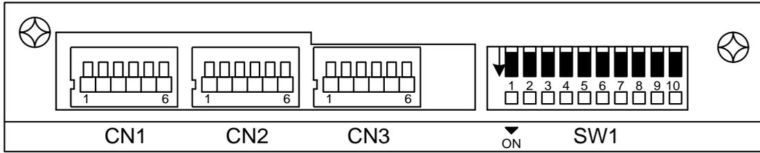
Fig. 9-1. Standard Board Connector and Dip Switch
