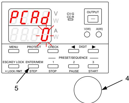
4. Turn the rotary encoder to change the value. The value range is from "0" to "31".
