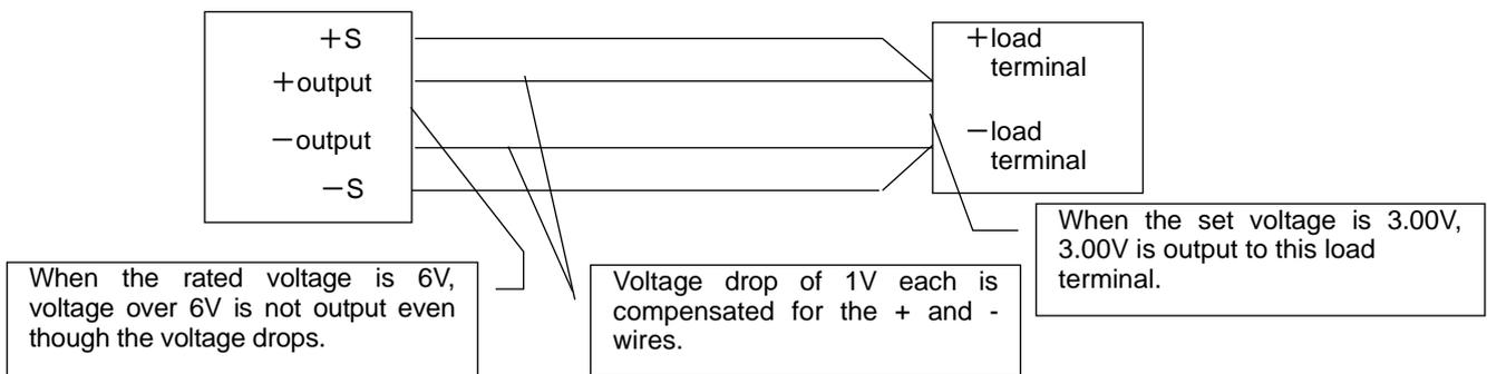
Fig.9 Connection with Load when Using Remote Sensing Function
