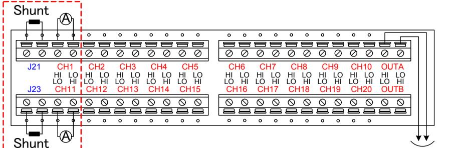
Note 1: CH1 & CH11 can be used on other measurement when the shunts are released from J21 & J23
