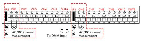
Note 1: CH1 & CH6 can be used on other measurement when the shunts are released.
