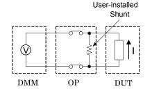
When the current shunts are installed, the channels will be limited to the current measurement unless users release the shunts.
