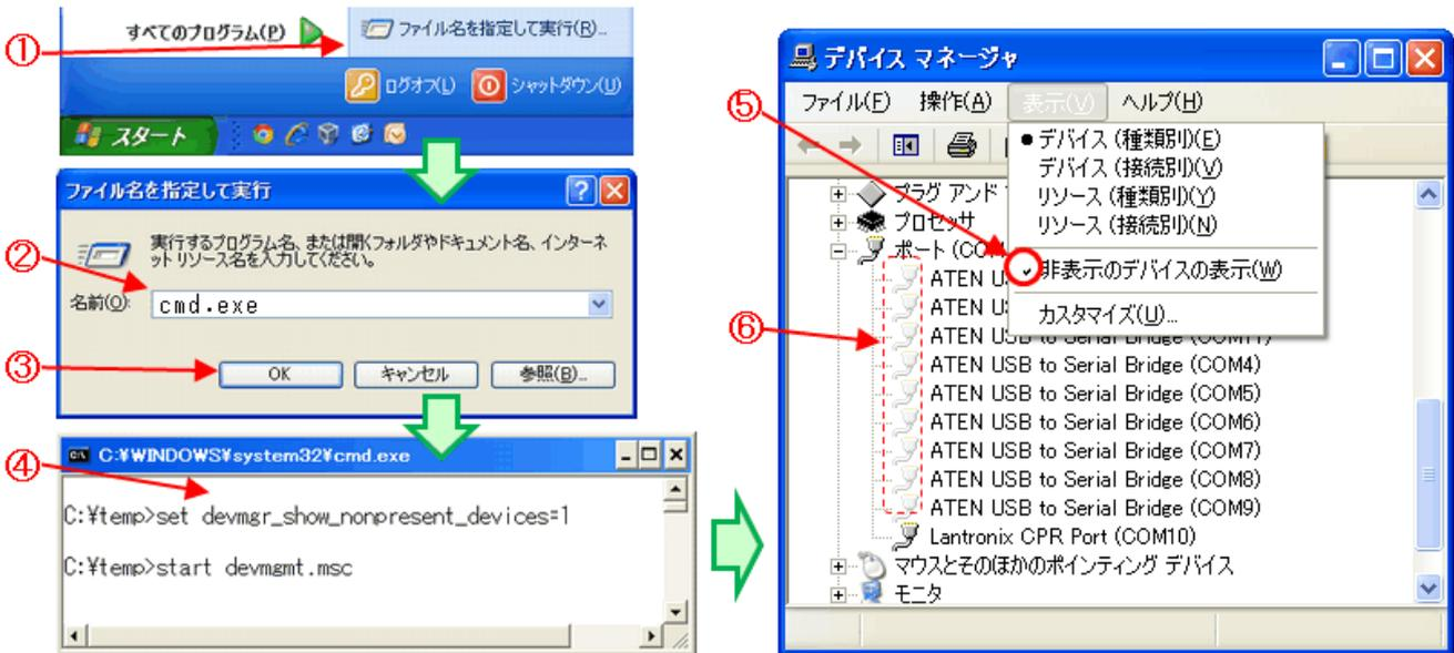
Fig. 4-7: Using Device Manager to display unconnected devices
