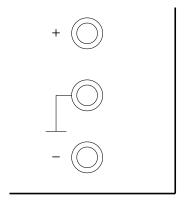
Connect the shorting bar between the + and GND terminals, or disconnect the GND cable as shown on the right. Disconnect the shorting bar.
