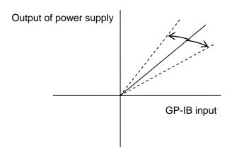
Set the FS output voltage (current) of the power supply units to be controlled through the GP-IB bus, and adjust the FS values with the semi-fixed variable resistors on the GP-600B panel. The FS variable resistor of each output has COARSE and FINE controls.
