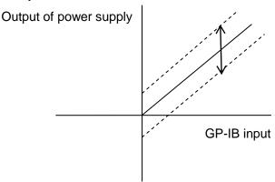
Set 1% output of the FS voltage (current) through the GP-IB bus, and adjust the offset so that output of the controlled power supply becomes 1% of the FS voltage (current) with the semi-fixed 0V control of each channel on the GP-600B panel.
