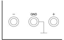
Connect the shorting bar between the - and GND terminals, or disconnect the GND cable as shown on the right.
