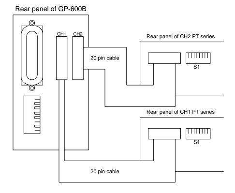
Use the OP-18-PT to connect the PT series with the GP-600B. Connect the 20-pin connector with the GP-600B and 26-pin connector with the PT series.
