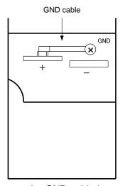
Connect the GND cable between the + and GND terminals, or disconnect the GND cable as shown on the right.
